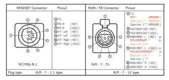
Note that the **MONI/TB** connector pinout varies, depending on the setting of the monitor switch.
