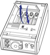
Note the two power indicators, one of which is lit when the unit is turned on, depending on whether battery power (**INT**) or DC power (**EXT**) is being supplied to the unit.
